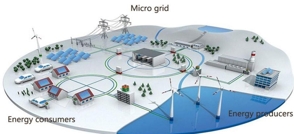
At its core is an energy storage system, which, through voltage and band management, achieves stable and quality power supply, renewable energy generation and management. The storage system facilitates peer-to-peer energy transfer (i.e. consumers can purchase stored energy contributed by prosumers). Combining IOT facilities that meet measurement requirements and technology standards of multiple countries for measurement and
